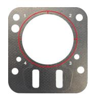
using a micrometer. Readings are taken from inside the cylinder hole of the gasket closest to the combustion chamber (see diagram). Four measurements are to be taken in the four defined quadrants with 3 meeting the minimum thickness of .042" (1.067mm).
