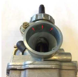
Both idle and main jet must remain stock, as shipped from the factory. Drilling of jets is not permitted.
